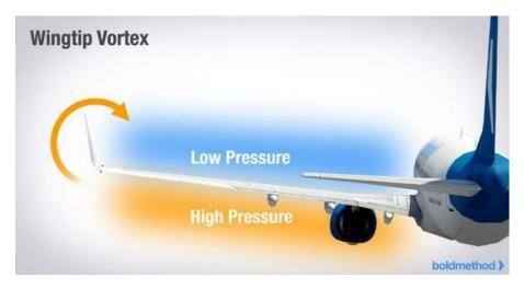
Figure 7: How wing tip vortexes are formed [12].
